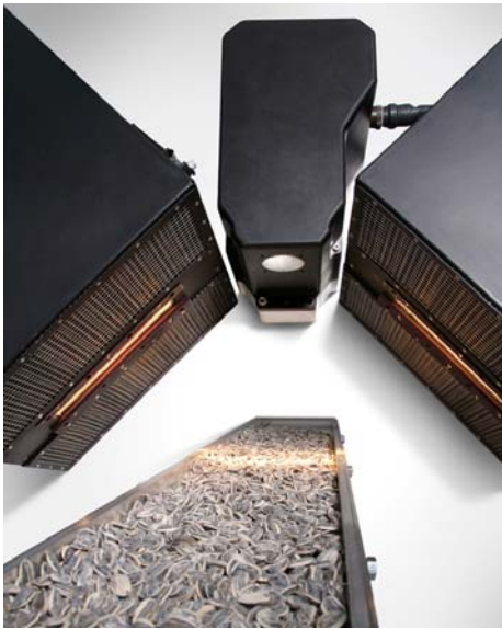
The INO camera with its illumination system
