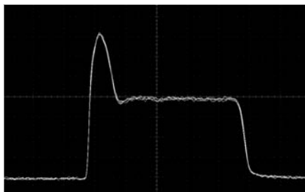
NANOSECOND PULSES WITH MULTI-KW OUTPUT PEAK POWER AND TAILORED SHAPES
