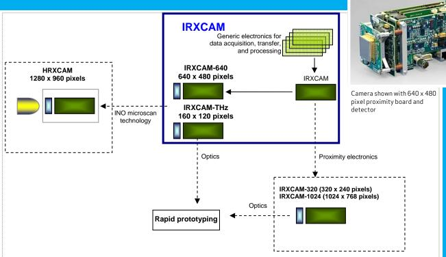
The IRXCAM main module is composed of a set of electronic boards that handle raw data acquisition and processing, final data formatting, synchronization with an external source, and data transfer according to various standards. The module is equipped with a Gigabit Ethernet link for a computer. The FPA is mounted on proximity electronics that are adaptable to various FPAs.
